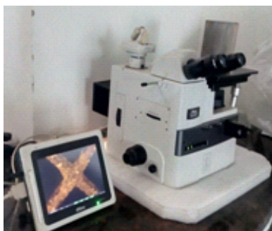
Fig. 1: Monolith substrate placed in inverted metallurgical microscope.
