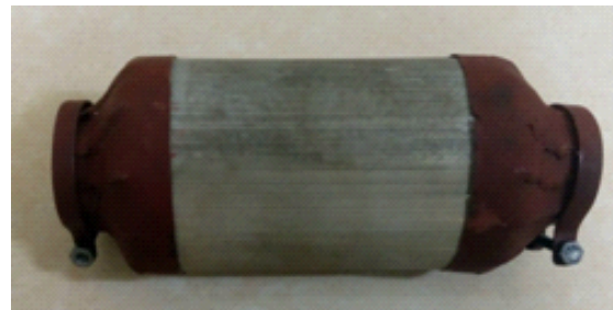
Fig. 11: Fabricated DOC with inlet and outlet lofts.
